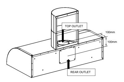
If the top outlet exhaust option has been selected, but the ducting routes through a wall to the rear, then the installation will require 215mm minimum head room in order to achieve a smooth 90° bend using 150mm flexible ducting.
