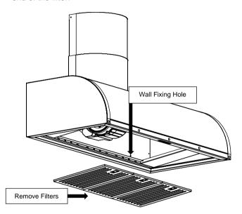
Once the filters have been removed, locate the wall fixing holes located at the rear bulk head of the appliance.
