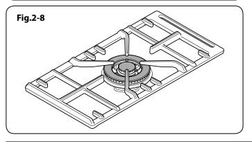
The igniter should spark and light the gas. Keep holding the knob pressed in to let the gas through to the burner for about ten seconds.
