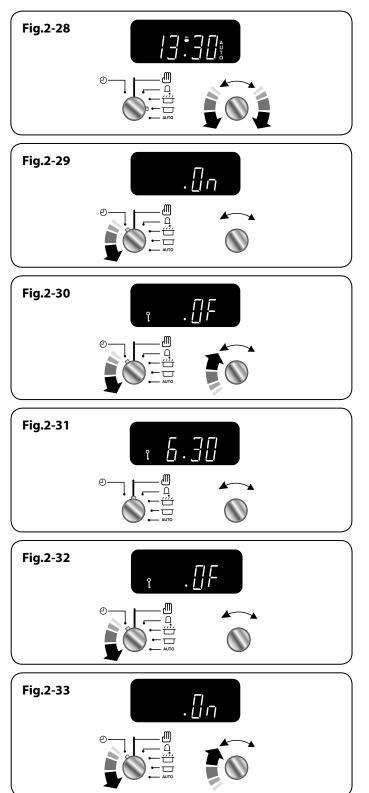
Turn the Timer knob to the  $[\Box]$  position. The display will show the current time of day plus the *'cook time'* you just set. Use the Adjusting knob to set the *'stop time'* required **(Fig.2-28)**.
