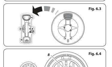
A – Electrode notch, B – Ignition electrode
