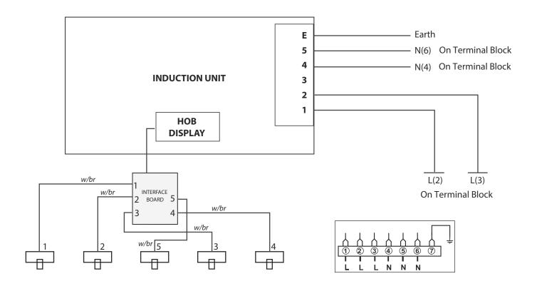
**Key**The connections shown in the circuit diagram are for single-phase. The ratings are for 230 V 50 Hz.
