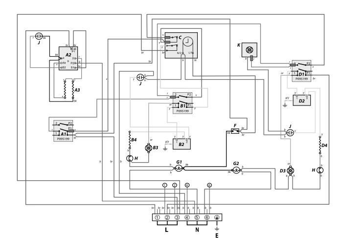
The connections shown in the circuit diagram are for single-phase. The ratings are for 230V 50 Hz.
