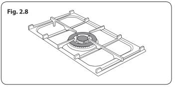
If, when you let go of the control knob, the burner goes out, then the FSD has not been bypassed. Turn the control knob to the OFF position and wait for one minute before you try again, this time making sure to hold in the control knob for slightly longer.
