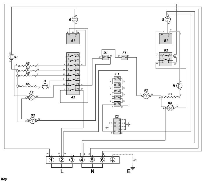
The connections shown in the circuit diagram are for single-phase. The ratings are for 230 V 50 Hz.
