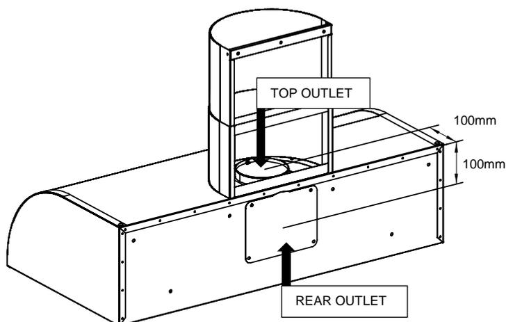
If the top outlet exhaust option has been selected, but the ducting routes through a wall to the rear, then the installation will require 215mm minimum head room in order to achieve a smooth 90° bend using 150mm flexible ducting.
