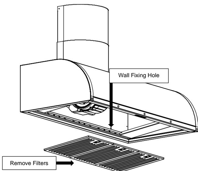
Once the filters have been removed, locate the wall fixing holes located at the rear bulk head of the appliance.
