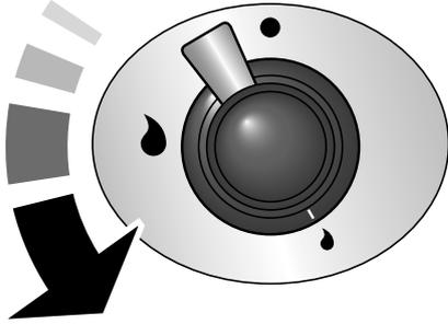
The igniter should spark and light the gas. Keep holding the knob pressed in to let the gas through to the burner for about ten seconds.
