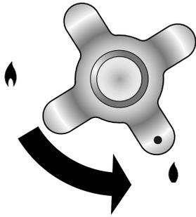
The igniter should spark and light the gas. Keep holding the knob pressed in to let the gas through to the burner for about ten seconds.
