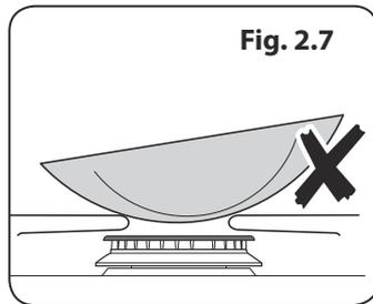
The minimum recommended pan diameter is 120 mm. The maximum allowable pan base diameter is 260 mm.
