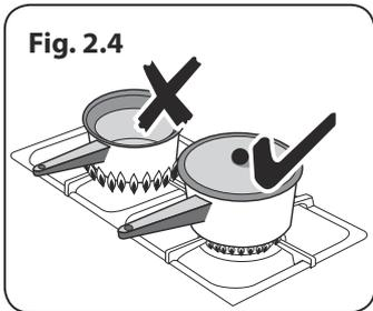
Make sure that the flames are under the pans. Using a lid will help the contents boil more quickly (**Fig. 2.4**).
