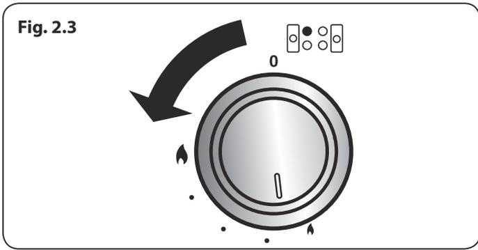
If and when you let go of the control knob or the burner goes out, then the FSD has not been bypassed. Turn the control knob to the OFF position and wait for one minute before you try again, this time making sure to hold in the control knob for slightly longer.
