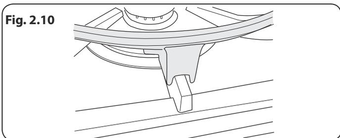
The cradle should be used on the wok burners only. When you fit the cradle, check that it is supported properly on a pan support and that the wok is sitting level in the cradle (**Fig. 2.10**).
