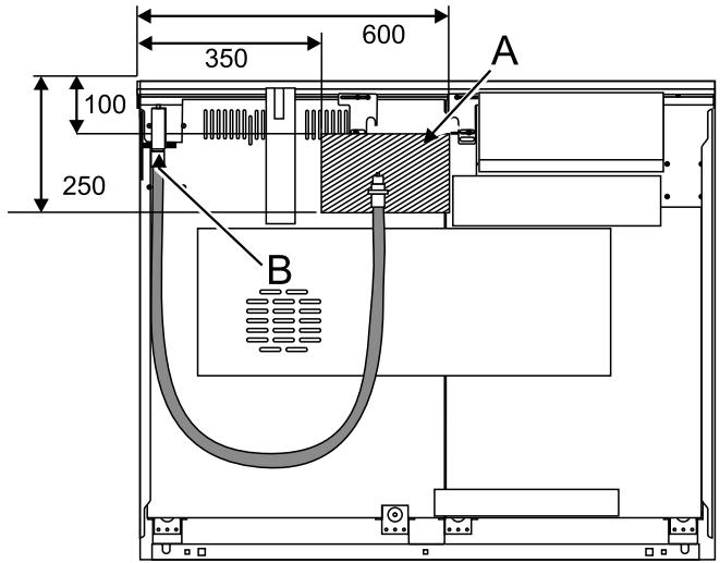
The rear cover boxes limit the position of the supply point. The house gas supply needs to terminate with a down facing connection.
