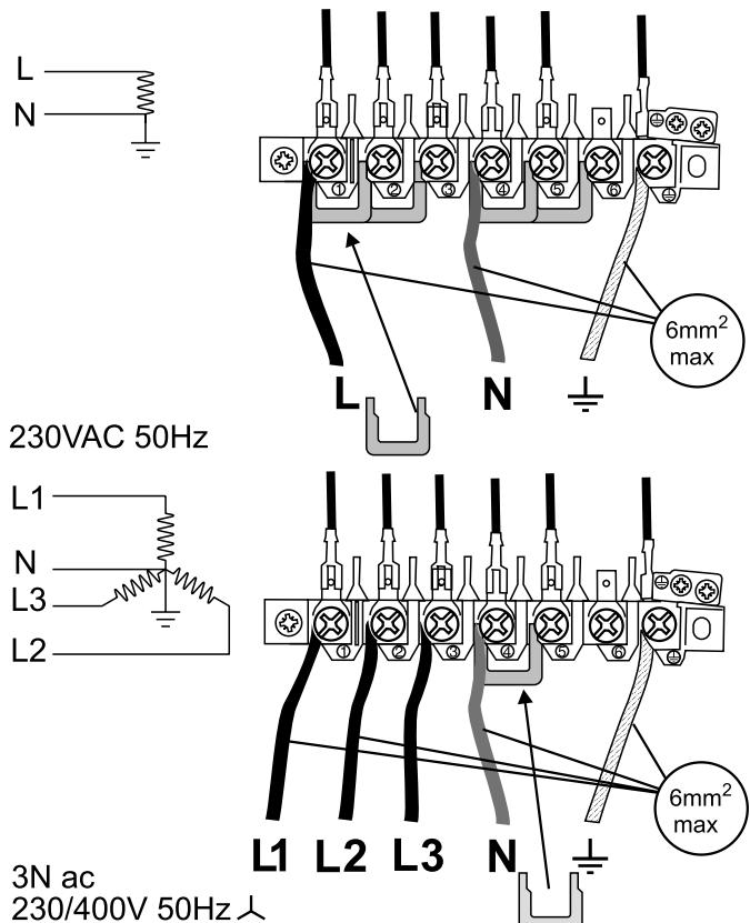
Check that the links are correctly fitted and that the terminal screws are tight. Secure the mains cable using the cable clamp.
