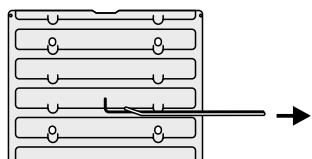
Lift up the front of the shelf so the back of the shelf will pass under the shelf stop and then pull the shelf forward.
