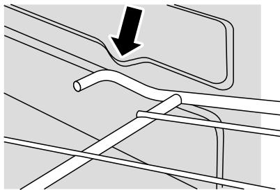
To refit the shelf, line up the shelf with a groove in the oven side and push the shelf back until the ends hit the shelf stop. Lift up the front so the shelf ends clear the shelf stops, and then lower the front so that the shelf is level and push it fully back.
