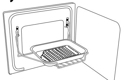
The Handyrack fits to the left hand oven door only. The maximum weight that can be held by the Handyrack is 5.5kg. It should only be used with the supplied meat tin, which is designed to fit the Handyrack. Any other vessel could be unstable.
