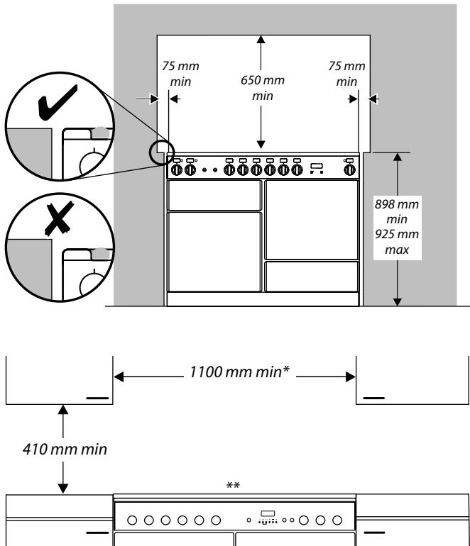
The hotplate surround should be level with, or above, any adjacent work surface. Above hotplate level a gap of 75mm should be left between each side of the cooker and any adjacent vertical surface.
