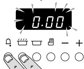
Press and hold as shown. At the same time, press (-) or (+) until the correct time shows. Don't forget it's a 24-hour clock. If you make a mistake or press the wrong button, turn off the power supply for a minute or two and start again.
