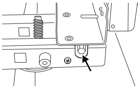
Adjust the height of the front roller to level the cooker. Turn clockwise to raise the cooker and anticlockwise to lower.
