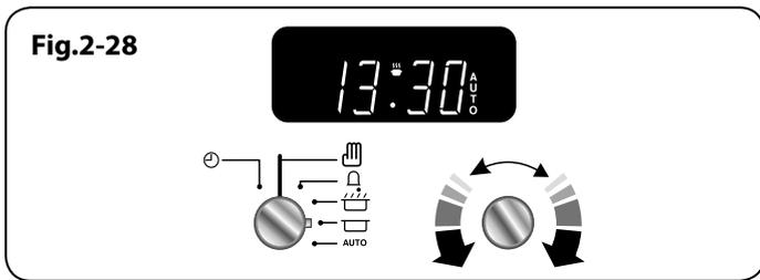
Turn the Timer knob to the [⌚] position. The display will show the current time of day plus the 'cook time' you just set. Use the Adjusting knob to set the 'stop time' required (**Fig.2-28**).
