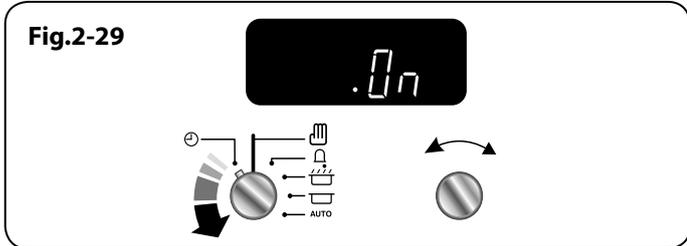
When your cooking is finished, the beeper sounds. Turn the Timer knob to the vertical [⏸] to return to manual cooking.
