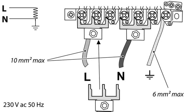
**Note:** The cooker must be connected to the correct electrical supply as stated on the voltage label on the cooker, through a suitable cooker control unit incorporating a double-pole switch, having a contact separation of at least 3 mm in all poles.
