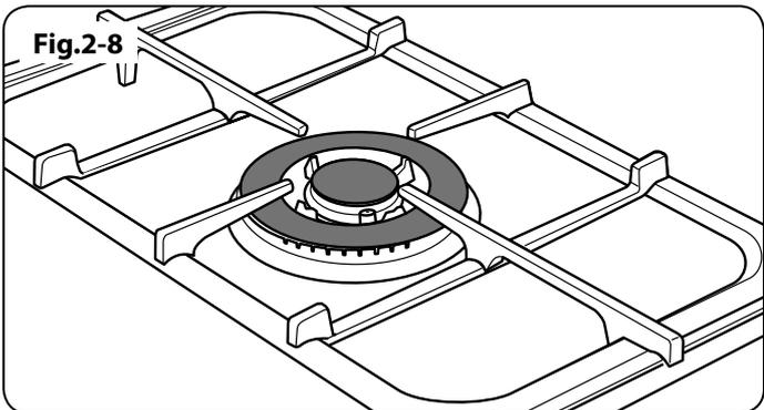
If, when you let go of the control knob, the burner goes out, then the FSD has not been bypassed. Turn the control knob to the OFF position and wait for one minute before you try again, this time making sure to hold in the control knob for slightly longer.
