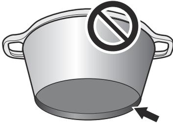
The minimum recommended pan diameter is 120 mm. The maximum allowable pan base diameter is 260 mm.
