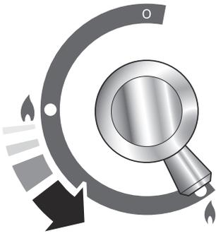
If, when you let go of the control knob, the burner goes out, then the FSD has not been bypassed. Turn the control knob to the OFF position and wait for one minute before you try again, this time making sure to hold in the control knob for slightly longer.
