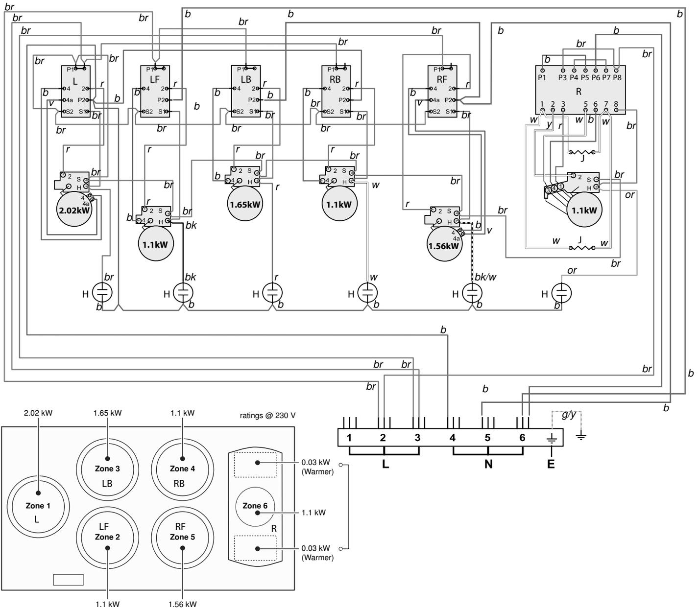
Connections shown in the circuit diagram are for single-phase. The ratings are for 230V 50Hz.
