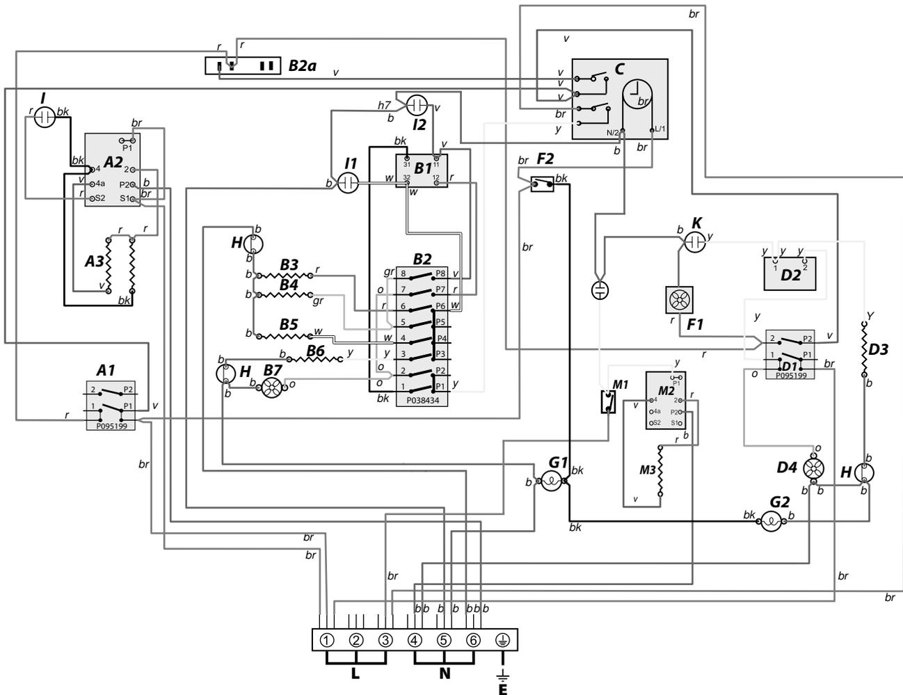
The connections shown in the circuit diagram are for single-phase. The ratings are for 230V 50Hz.
