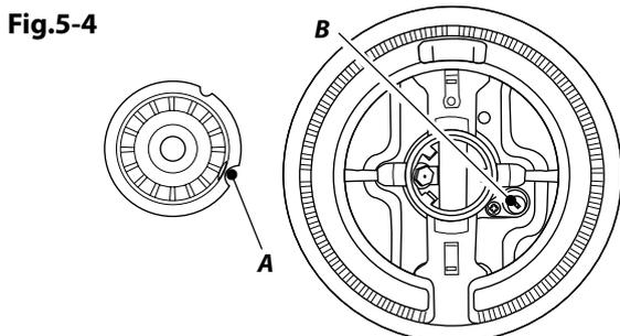
A – Electrode notch, B – Ignition electrode
