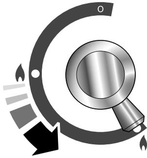
If, when you let go of the control knob, the burner goes out, then the FSD has not been bypassed. Turn the control knob to the OFF position and wait for one minute before you try again, this time making sure to hold in the control knob for slightly longer.
